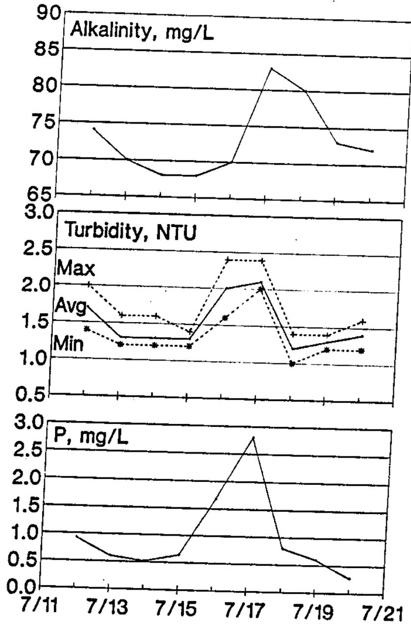
Figure 24. Secondary Effluent Alkalinity, Turbidity and Phosphorus Forms, July 1989
