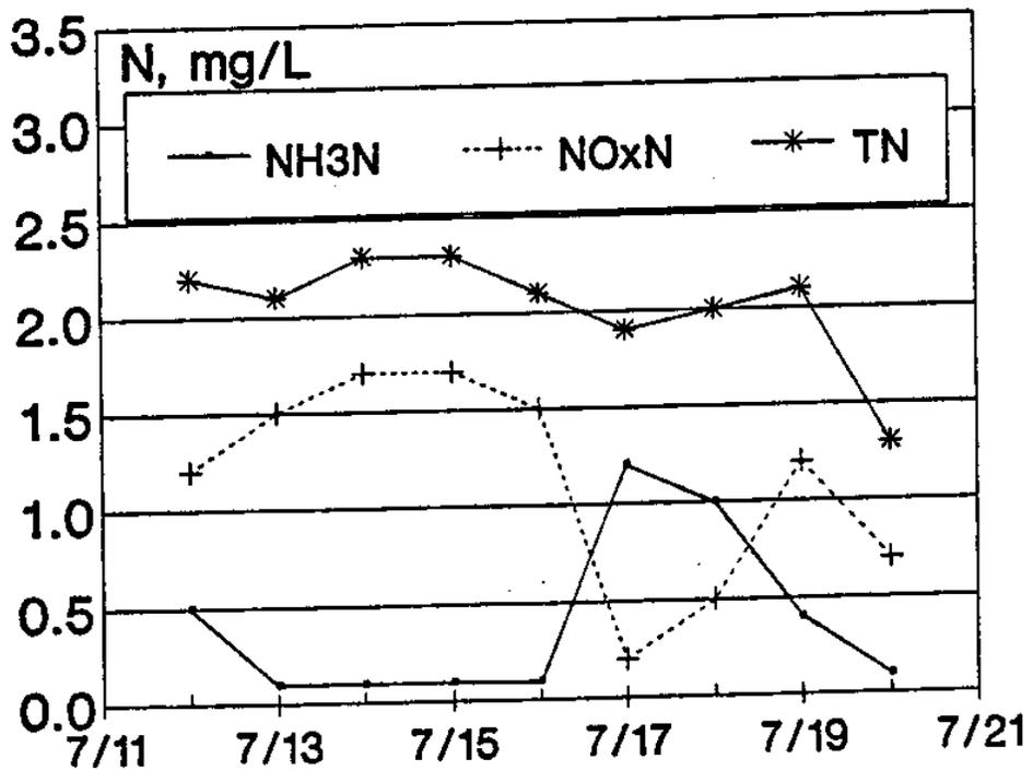
Figure 23. Secondary Effluent Alkalinity and Nitrogen Forms, July 1989
