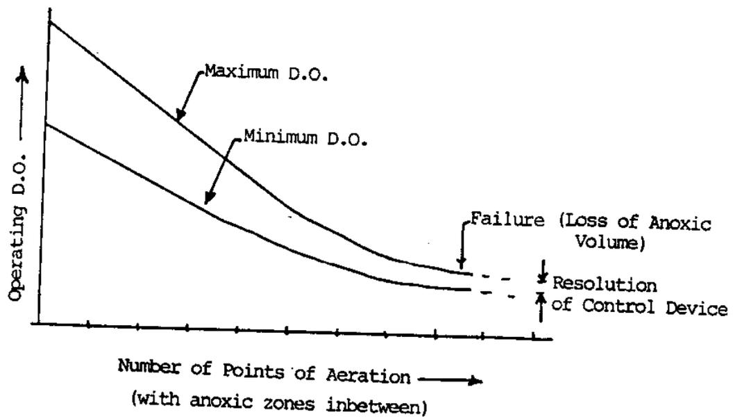
Figure 17. Minimum and Maximum Operating D.O. plotted against Number of Points of Aeration
