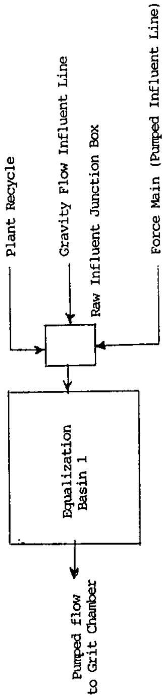
Figure 2. Schematic of Raw Influent Junction Box
