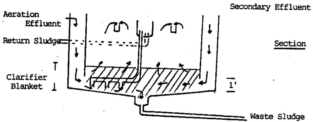
Figure 3. Schematic of Secondary Clarifier
