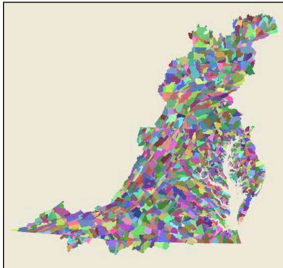
Figure 7-1: Scale of Watershed Model-HSPF Phase 5 Output. Each segment has up to 25 land uses.
