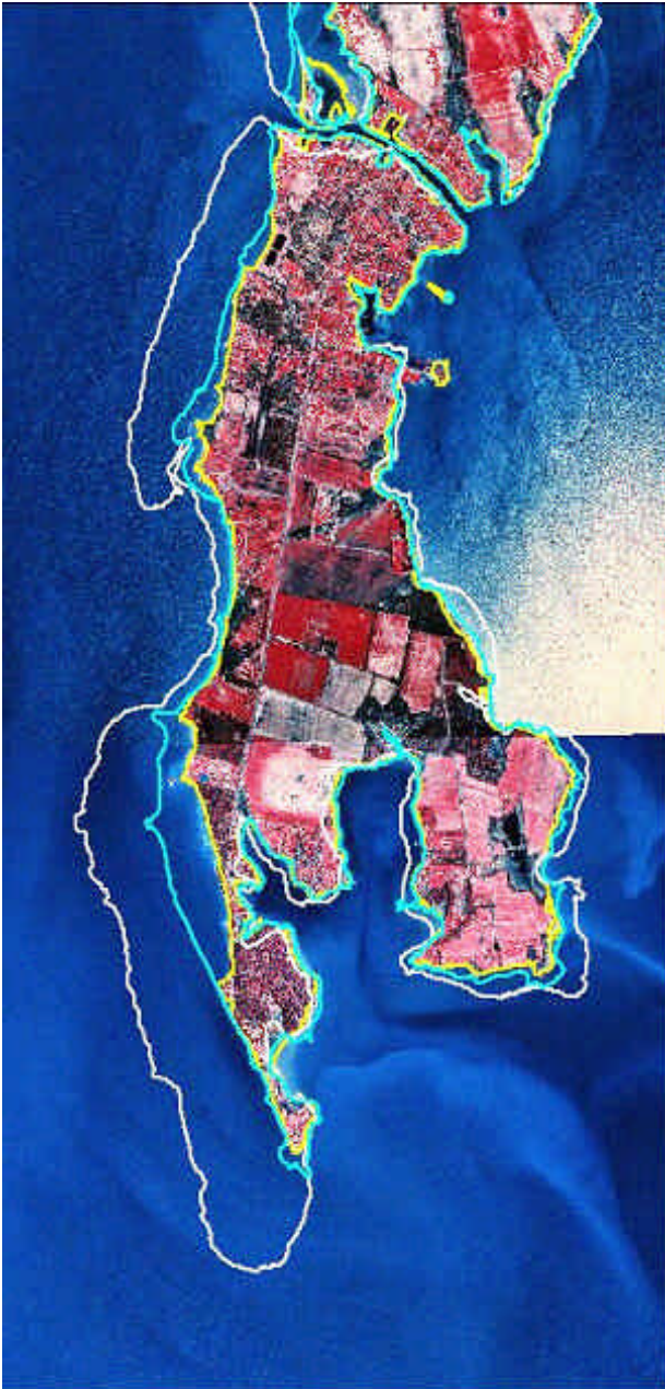
Figure 1. Example of changing shorelines at Tilghman Island, Maryland overlaid on a 1989 color infrared photograph of the island. The white line indicates the shoreline position in 1842, the blue in 1945 and the yellow in 1989. (Source: Maryland Geological Survey)
