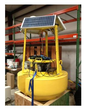
Oceanographic buoys that can be paired with acoustic receivers and generate synoptic and realtime data on habitat and fish location, e.g.
