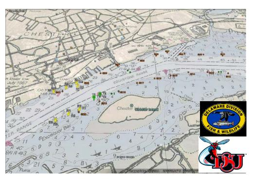
VEMCO Positioning System (**VPS**) array that combines passive deployment with better spatial precision
