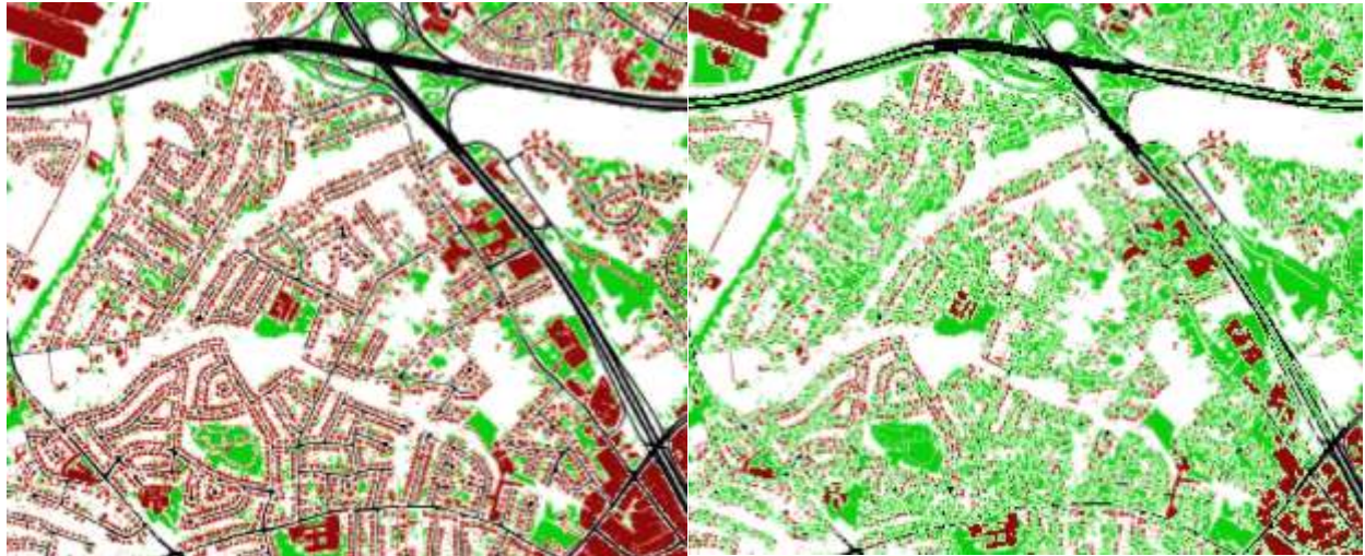
Figures 8 & 9. Ten-meter resolution land cover data using the same extent as shown in Figure 7. In the left image, the order of the overlay from top to bottom is: roads (black), other impervious (red), and low vegetation (green). In the right image, the data were re-ordered with low vegetation moved on top of roads and other impervious surfaces.
