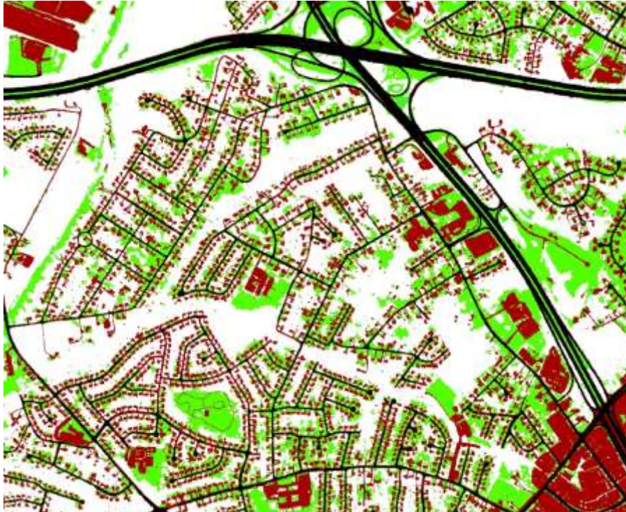
Figures 6. High-resolution (1-m) representation of roads (black), other impervious surfaces (red), and low vegetation (green).
