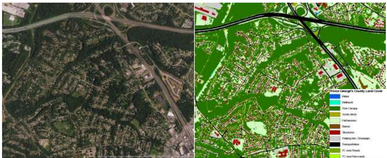
Figures 3 & 4. Example of a recent high-resolution aerial image (left) and 2013 classified land cover dataset (right) for an area in Prince George's County, Maryland.
