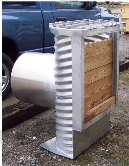
Figure STTL.3. Flashboard Dam Dewatering Device (forums.pondboss.com)
