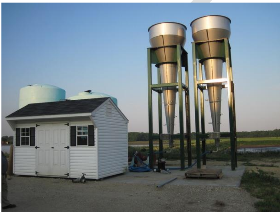
Figure WCT.5. Demonstration of the Latest Generation of Cone Struvite Crystallizer on a Dairy Farm near Massey, Maryland (Sassafrassriver.org).
