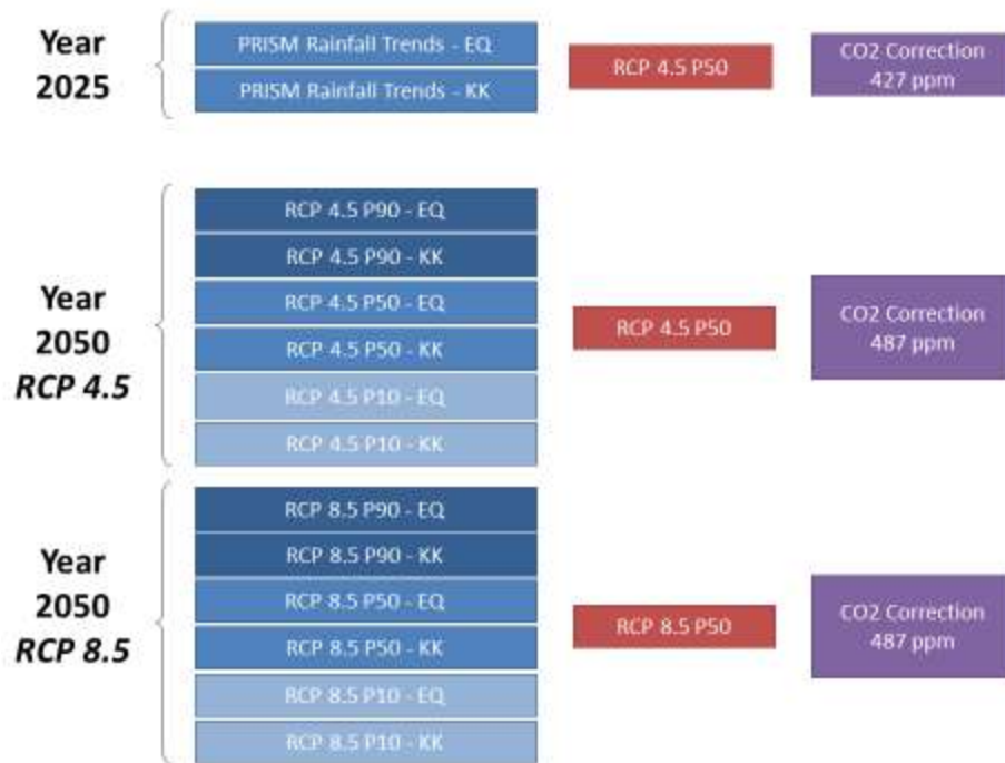
Figure 1. The 14 climate scenarios now being developed for the 2025 and 2050 future conditions (with RCP 2.6 scenarios to be added). All scenarios have either the estimated increased precipitation volume added evenly throughout the time series of precipitation events (EQ) or increased volume assigned to different percentiles of precipitation events as described by Groisman, Pavel Ya, et al (2004). The 2050 scenarios were developed by determining the median, 10 th percentile, and 90 th percentile of altered precipitation volumes from an ensemble of downscaled GCMs defined by the guidance presented in the U.S. Climate Resilience Toolkit.
