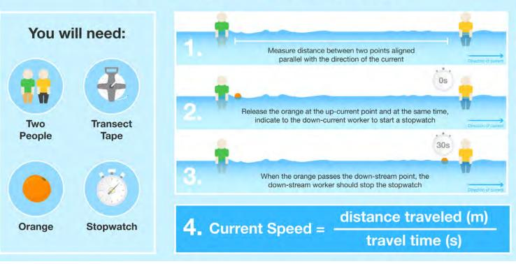
Figure 18 - A simple method to estimate water velocity.
