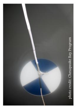
Figure 13 - Secchi disc being lowered into the water to determine water clarity.
