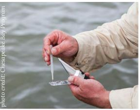
Figure 17 – Using a dropper to place a water sample on a refractometer to measure salinity.
