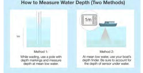
Figure 12 - Two methods for measuring water depth at your potential restoration site.
