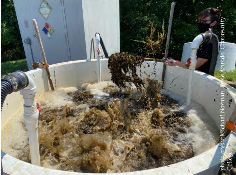
Figure 32 - Harvested material being processed in the Turbulator. Redhead grass shown here.
