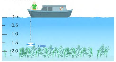
Figure 14 - How to use a Secchi disc to measure water clarity.
