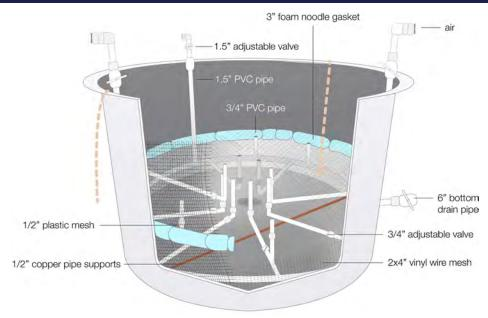
Figure 29 - Schematic of the Turbulator.
