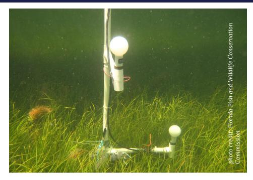
Figure 15 - A light profiler deployed in an SAV bed.
