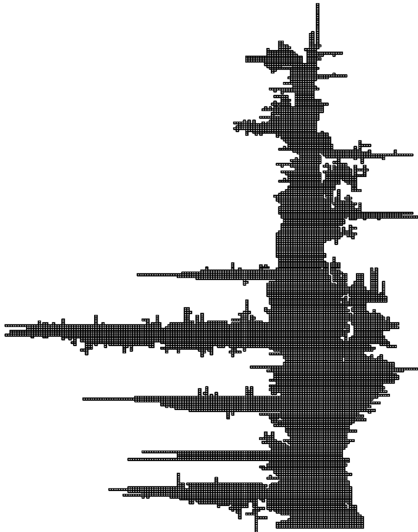
Figure 2. Rectilinear plan view of 50,000-cell CH3D Chesapeake Bay grid. In this view, all cells are represented as unit squares. This view emphasizes the number of cells in narrow reaches such as the tidal freshwater portions of the tributaries.
