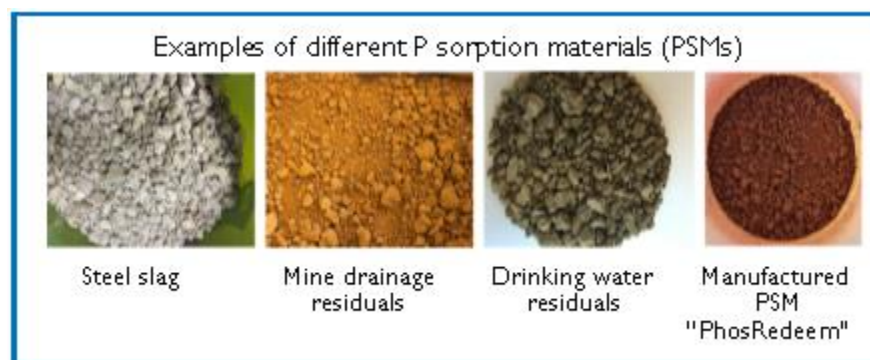
Figure 10. Examples of several P sorption materials (PSMs)
