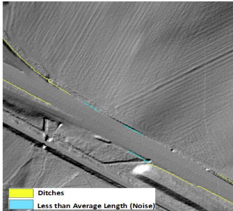
Figure 10. Illustration of average length criteria used to distinguish ditches from noise
