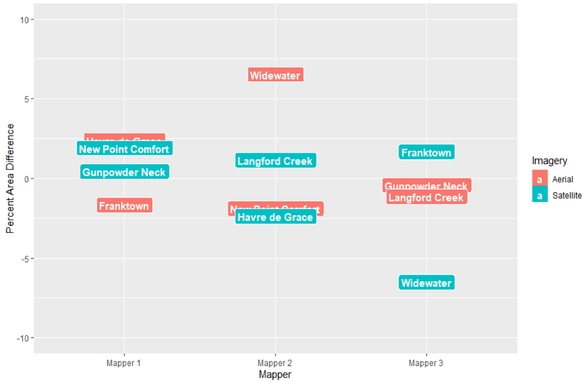
Figure G-4. Percent area difference from the mean for the aerial and satellite interpreted versions of each USGS quadrangle comparison area by each mapper. Results show that no mappers exhibited a consistent bias toward one imagery type or the other.
