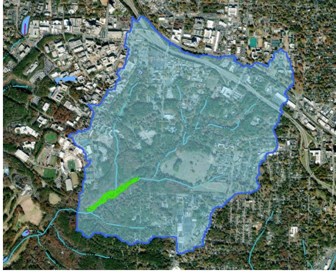
Figure 16. Sandy Creek watershed (1.72 sq. mi.) shown in blue and the floodplain area (8.1 acres) associated with the Sandy Creek Phase I stream restoration project show in green.
