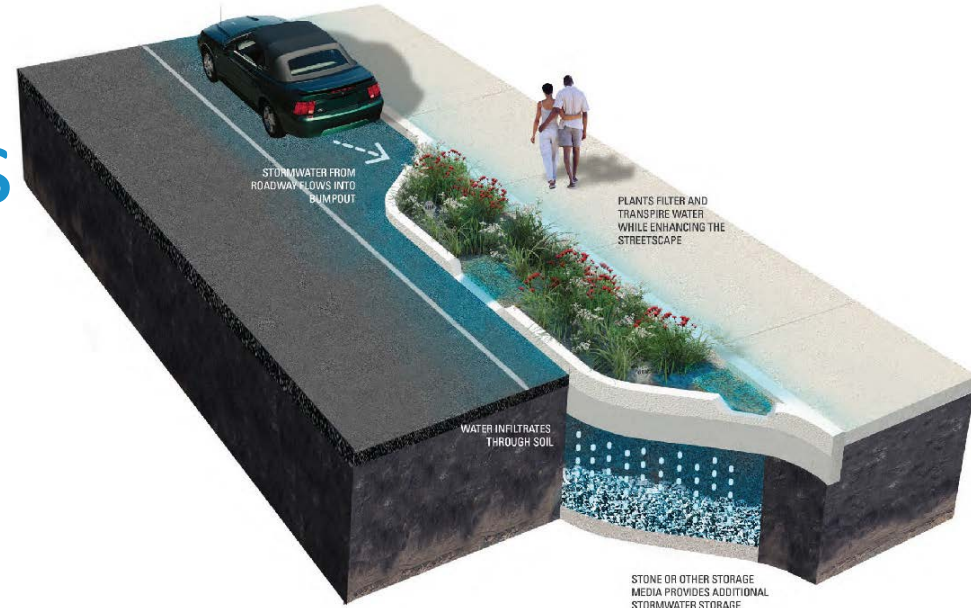
Mid-block Stormwater Bump-out
