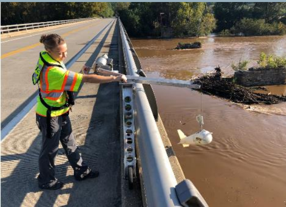
Above: A hydrologic technician collects a water-quality sample from the Chesapeake Bay nontidal monitoring network (NTN) following a large storm, conditions often transport elevated bacteria counts.
