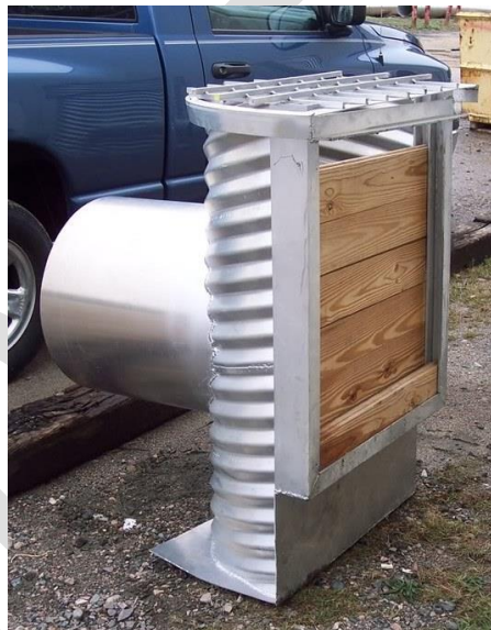
Figure STTL.3. Flashboard Dam Dewatering Device (forums.pondboss.com)
