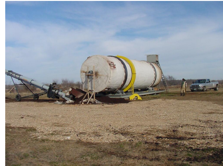
In-Vessel (Rotating Bin)
