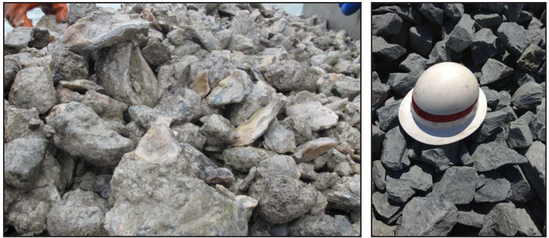
Figure 21: Photos of fossil shell substrate (left, DNR, 2014) and stone substrate, with hard hat shown for scale (NOAA, 2014).
