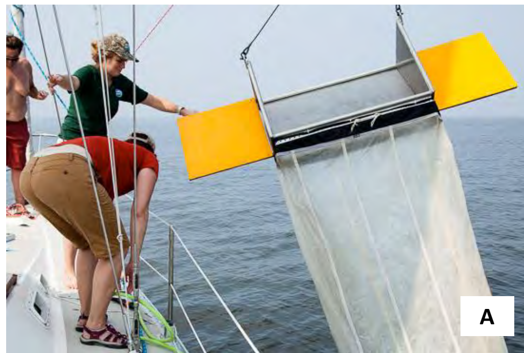
Figure 1 – (A) Sampling for microplastics with manta trawl in Chesapeake Bay; (B) Microplastics collected from the Magothy River (Photos: Will Parson, Chesapeake Bay Program Office)
