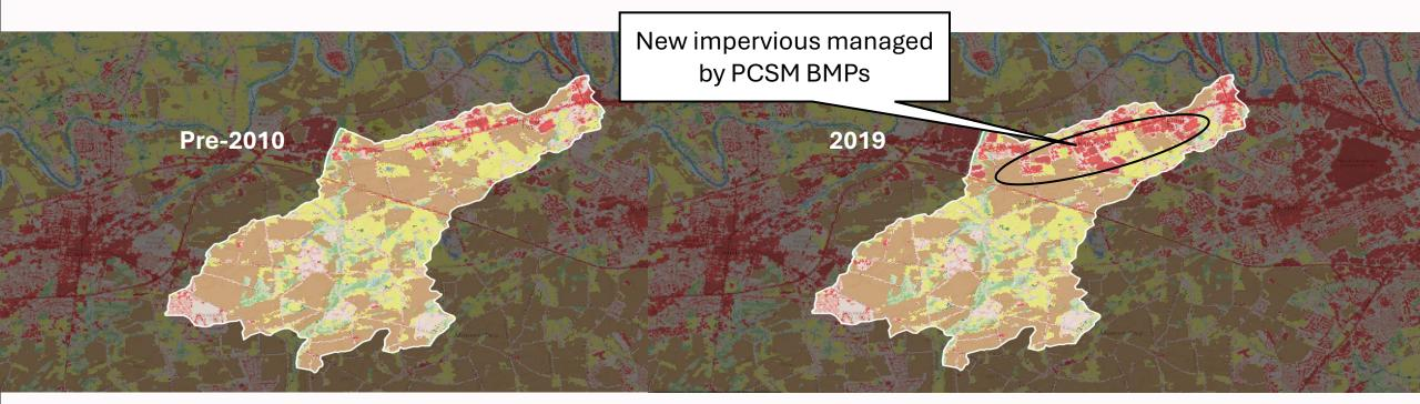
Because of the Construction NPDES permit requirements, we know that the majority of runoff from new impervious (implemented since 2010) is being managed by PCSM BMPs.
