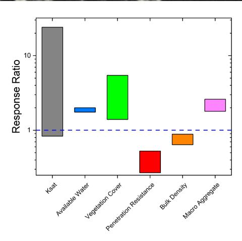
The range of response ratios for  $K_{sat}$  and related soil parameters for all sites except MDTA US-279. Data are based on measurements more than 1 year after 4% biochar incorporation.  $K_{sat}$  response ratio <1.0 indicates that biochar amendment decreased infiltration, observed at only one site where gravel was in the native soil but not in the biochar amended region. (Akpinar et al., 2023)
