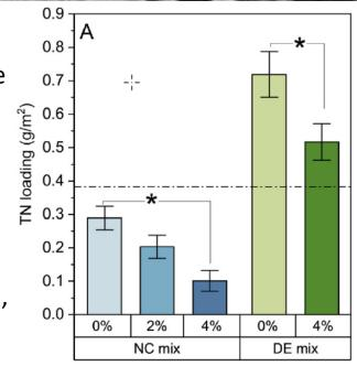
Effect of biochar amendment (0, 2, and 4% by mass) on total nitrogen (TN) loading from two bioretention media – NC mix (without compost) and DE mix (with compost). Influent TN loading is horizontal dashed line. Biochar amendment decreased TN loading from both media, although TN in DE mix exceeded influent when compost present. Taken with permission from Akpinar et al. (2023b).
