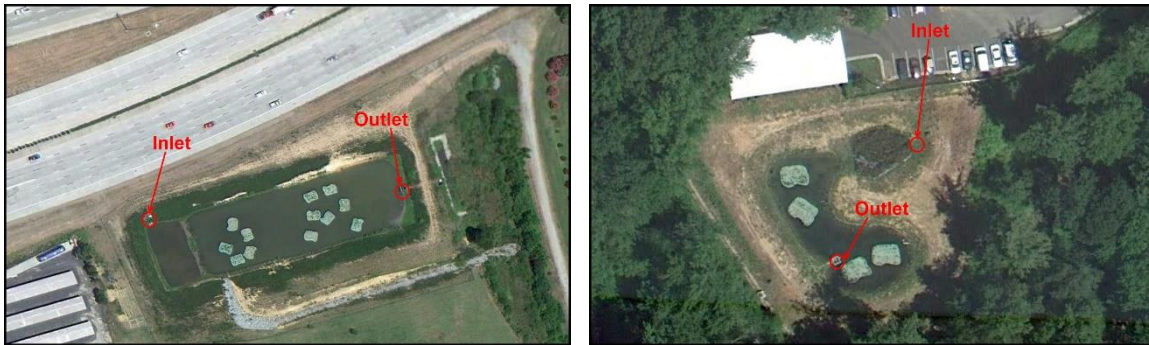
Figure 1. Overhead Shot of FTWs Deployed in Two North Carolina Wet Ponds (Winston et al, 2013)
