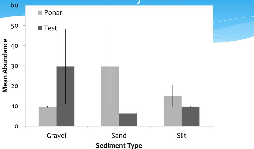
Ponar Grab vs. Test Grab (ANOVA, gravel p = 0.208, sand p = 0.457, silt p = 0.865)
