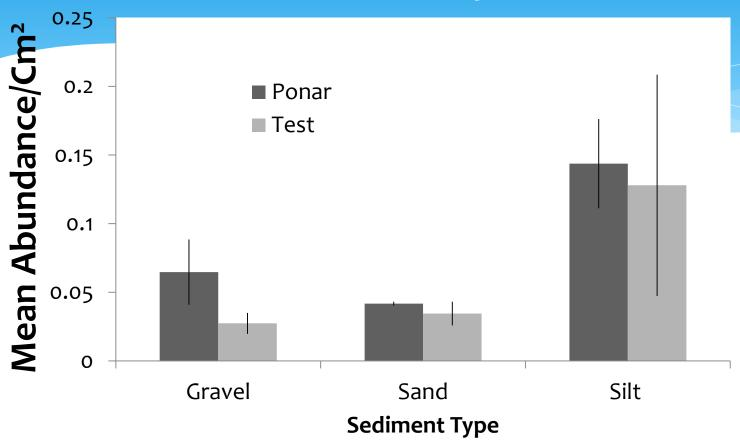
Comparison of mean abundance of organisms/cm<sup>2</sup> (ANOVA, gravel P=0.208, sand P=0.457, silt P=0.865) preliminary field sample.
