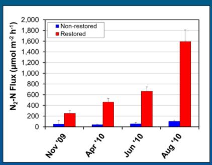
At this rate, if 23% of the suitable bottom in the Choptank River were restored with comparably healthy oyster reefs, it would equal the entire nutrient reduction target for that tributary.
