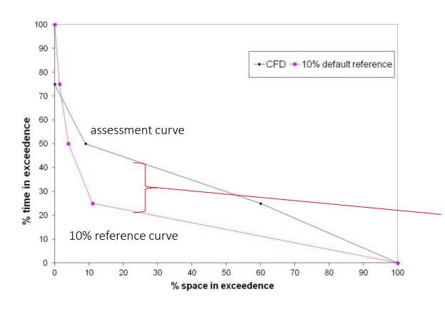
Area between the curves = excessive space-time exceedence rate
