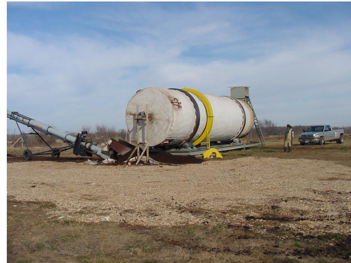
In-Vessel (Rotating Bin)
