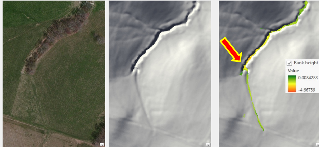
Example #1: Headcut identification
