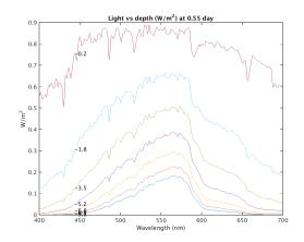
Short wavelengths reduced; long wavelengths strongly reduced.
