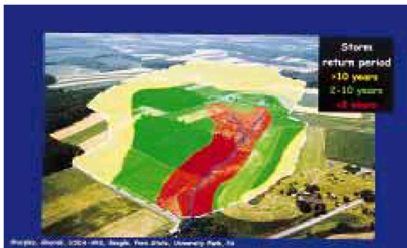
Figure 3. Surface runoff potential. Shows return periods of less than 2, 2 to 10 and greater than 10 years overlaid on the watershed.
