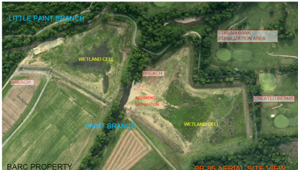
Figure 2. Floodplain Restoration by Raising the Stream Bed (Courtesy: Joe Berg, Biohabitats)
