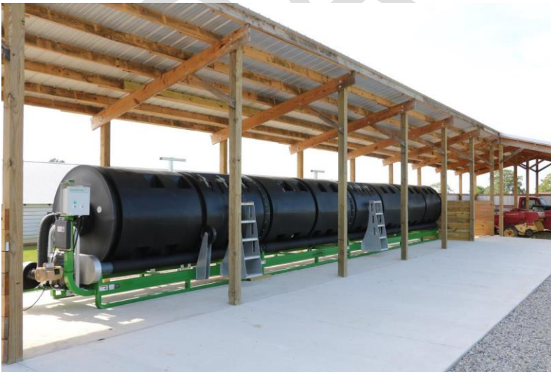
Figure II.3.6. Ecodrum™ rotating drum mortality composter (Mark Hutchinson).
